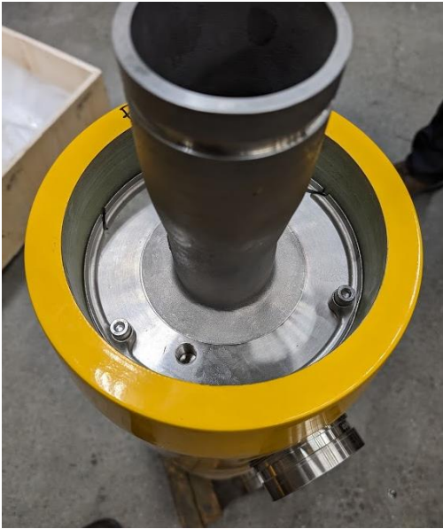
Figure 8-26 Assemble lock-ring and cap screw
